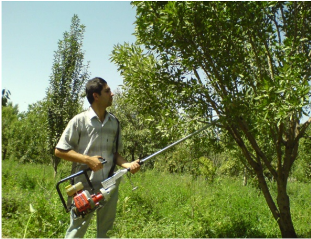
Fig 1. Limb shaker in operation
