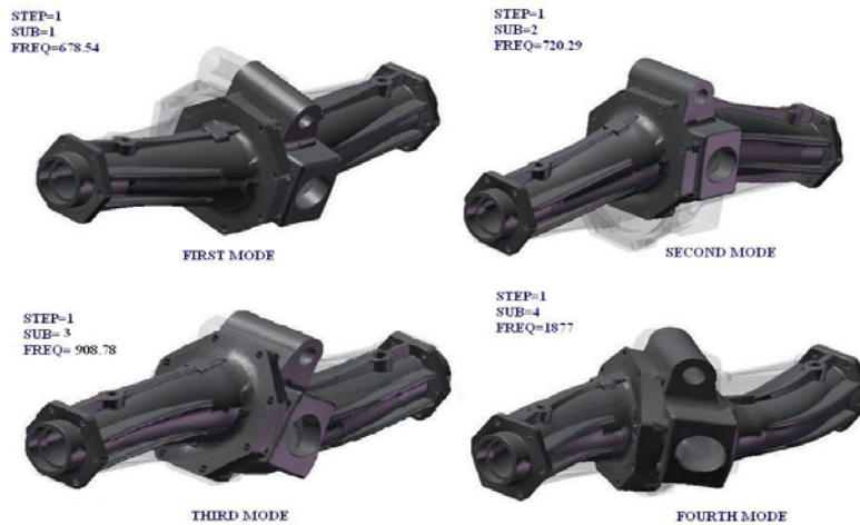
Fig 8. The first four mode shapes of housing
