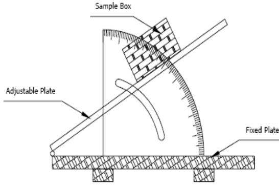
**Fig 1.** Schematic of apparatus for determining angle of repose
