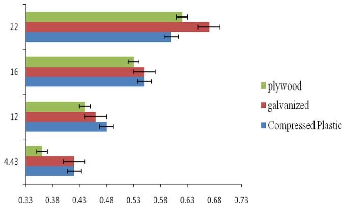
**Fig 4.** Effect of moisture content on the static coefficient of friction of sunflower against various surfaces
