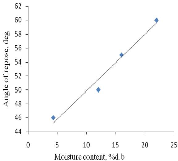
**Fig 5.** Effect of moisture content on angle of repose of sunflower seed (20 repeat for each moisture content)
